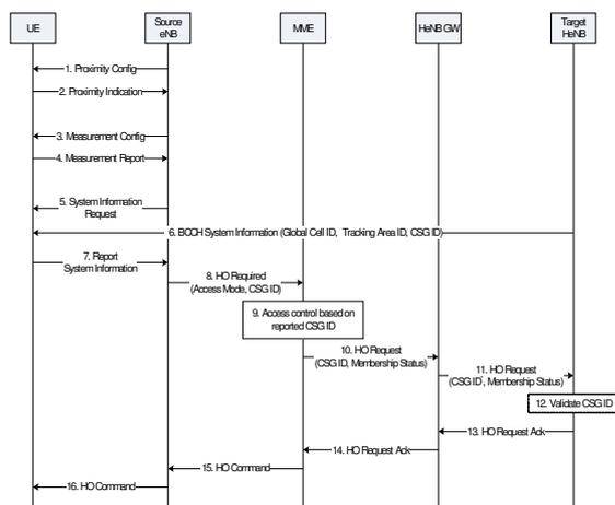
**Figure 2: Inbound Mobility to HeNB CSG and hybrid Cells**
